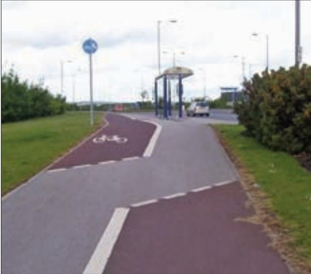
Figure 8.4 Cycle track changing sides at bus stop (Tim Pheby)
