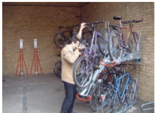
Figure 11.6 Spring-assisted stacking cycle rack (Tony Russell CTC)
