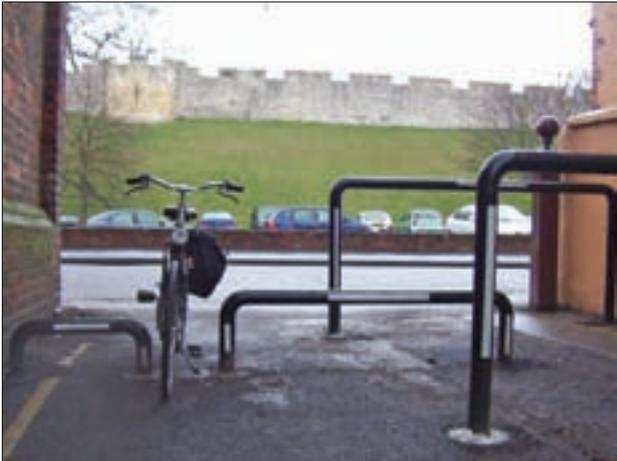
Figure 8.7 Barrier with wheelchair bypass (Tim Pheby)
