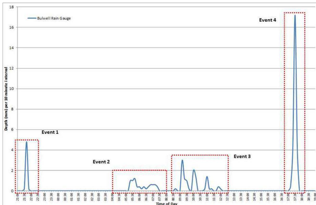
Figure 2: Rain gauge data from Bulwell for the evening of 22<sup>nd</sup> July 2013 and throughout 23<sup>rd</sup> July 2013
