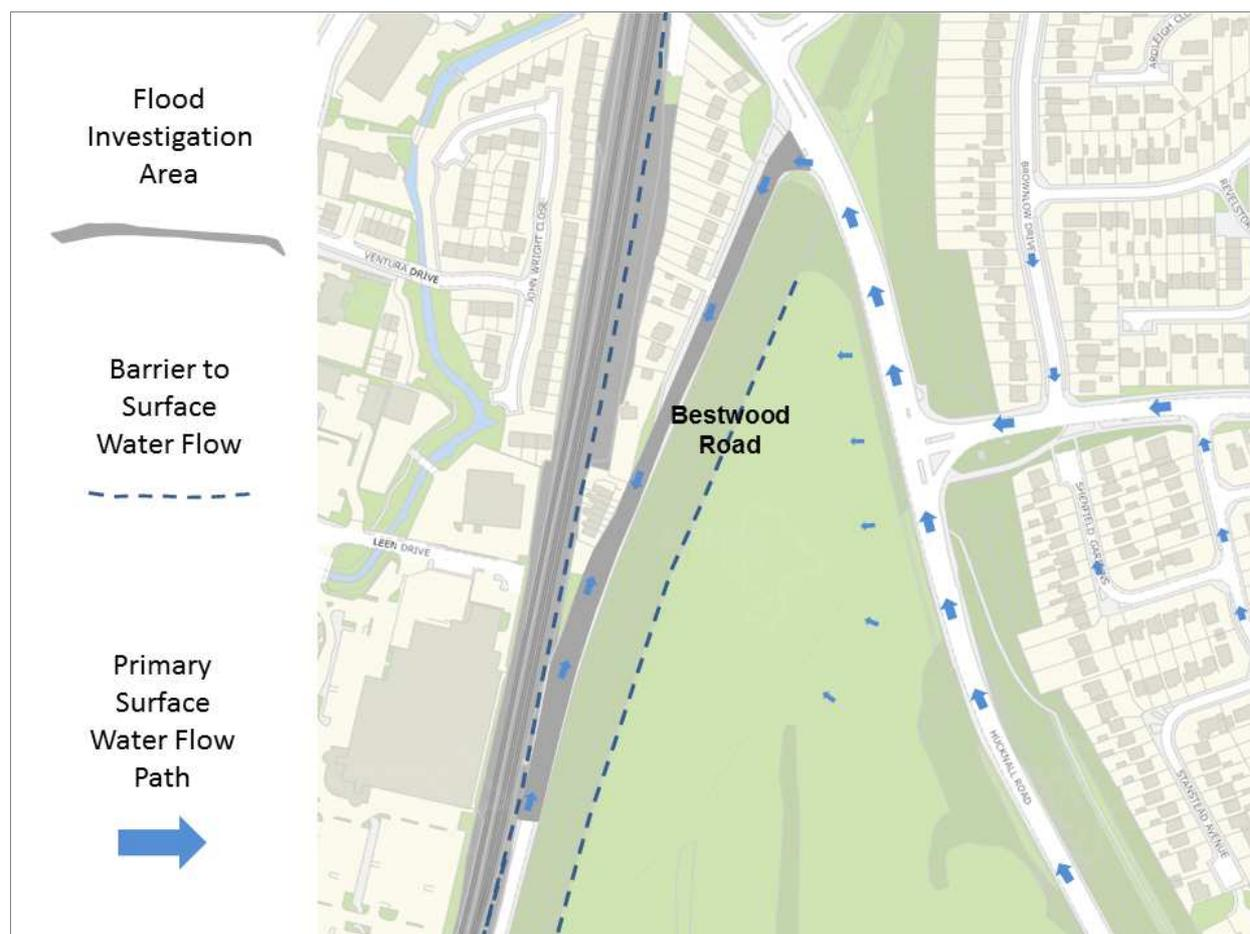
**Figure 3: Primary flow routes of surface water during the flood event (based on observed topography).**
