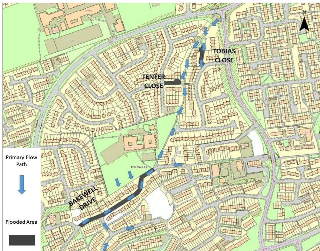
**Figure 3: Primary routes of surface water during the flood event.**
